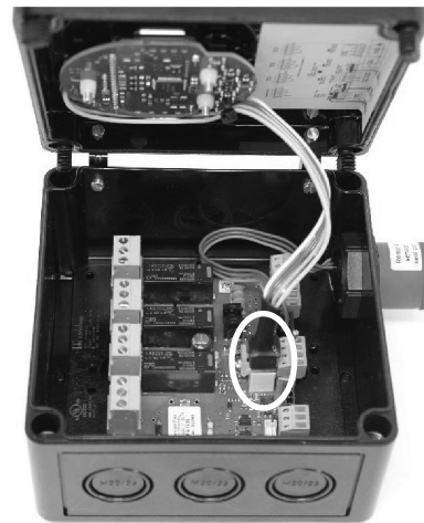
Figure 2: Unplug of the display PCB
