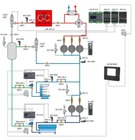
HP High Pressure (120-140 bar) HP Receiver Pressure (60-90 bar) LP Suction Pressure MT (45-55 bar) LP Suction Pressure LT (25-30 bar)
