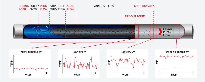
Danfoss Adaptive Minimum Stable Superheat Control (MSS)
