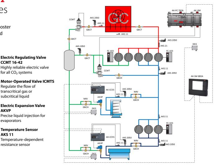
HP High Pressure (120-140 bar) HP Receiver Pressure (60-90 bar) LP Suction Pressure MT (45-55 bar) LP Suction Pressure LT (25-30 bar)
