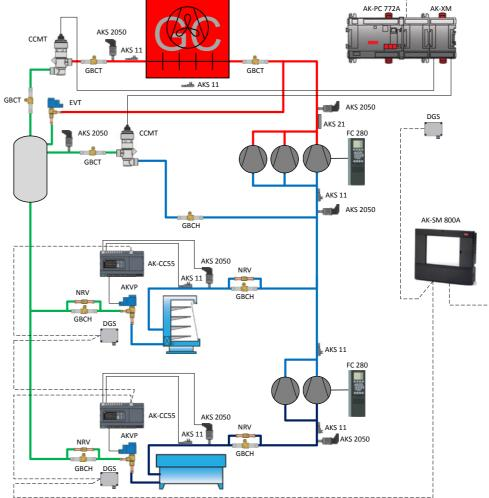
HP High Pressure (120-140 bar) HP Receiver Pressure (60-90 bar) LP Suction Pressure MT (45-55 bar) LP Suction Pressure LT (25-30 bar) **Electric Regulating Valve**
