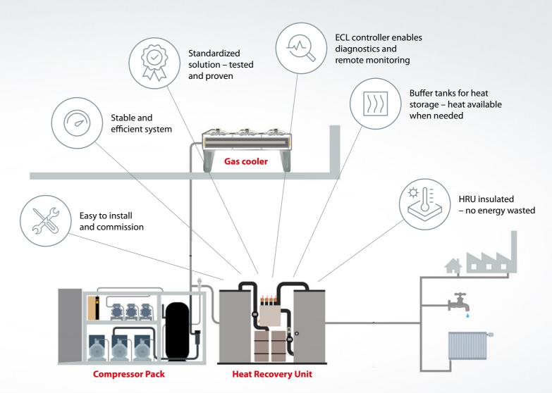
With an HRU unit, **get maximum heat recovered and reused** with no or minimum need for additional heat sources.
