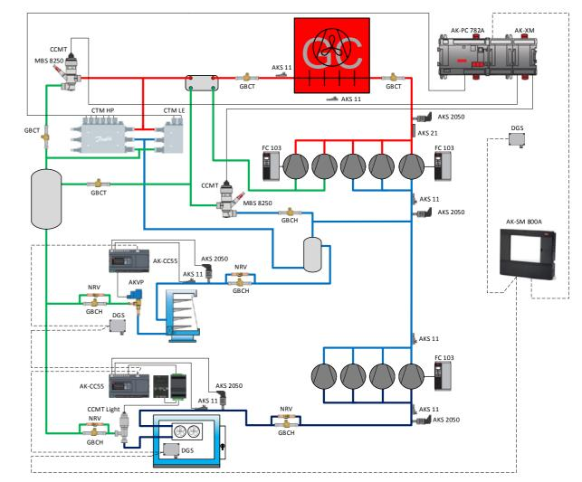
HP High Pressure (120-140 bar) HP Receiver Pressure (60-90 bar) LP Suction Pressure MT (45-55 bar) LP Suction Pressure LT (25-30 bar)
