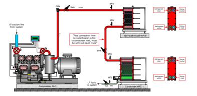
Liquid cooled Desuperheater (Heating of brine)
