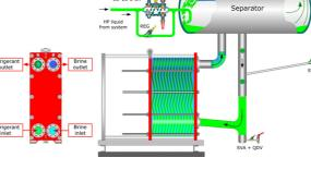
Liquid cooled Condensers (Heating of brine)
