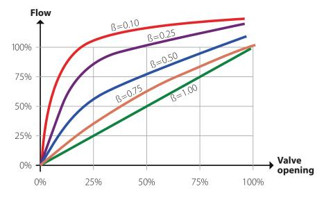
For conventional systems, increasing pressure across the control valve decreases valve authority ( $\beta$ ). The effect is nearly full flow for only a small valve opening.
