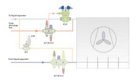
ICLX are used in wet return and suction lines for the opening against high differential pressure, e.g. after hot gas defrost in large industrial refrigeration systems with ammonia or fluorinated refrigerants.
