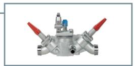
Suction line valve station with temperature control In this evaporator example you can replace the individual valves with an ICF 65-3 with SVA-S stop valve, ICS servo operated control valve and SVA-S stop valve. This ICF solution saves you 5 weldings in this application.
