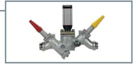
Hot gas line valve station with motor operated valve In this hot gas line example you can replace the individual valves with an ICF 50-4 with SVA-S stop valve, FIA strainer, ICM motor valve and REG-SB hand expansion valve. This ICF solution saves you 4 weldings in this application.
