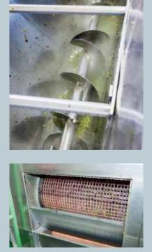
Once the grapes have been removed from the stems, they go to the scales and then into two eccentric screw pumps, which transport them to the presses, which squeeze the juice from the grapes. The juice then goes into tanks for fermentation.
