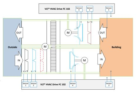
Example of installation: This air handling unit is equipped with 7 sensors. The inlet and outlet are controlled by separate VLT® HVAC Drives.
