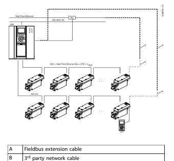
Illustration 2.5 Ethernet POWERLINK<sup>®</sup> with Redundancy via PLC
