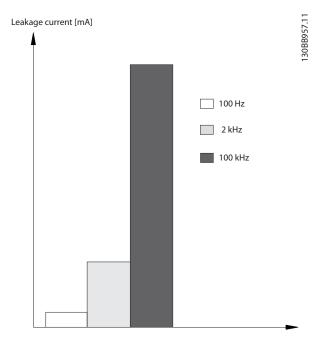
Illustration 4.4 Influence of RCD Cut-off Frequency on Leakage Current
