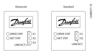
Illustration 2.19 Operating LEDs on the Servo Drive
