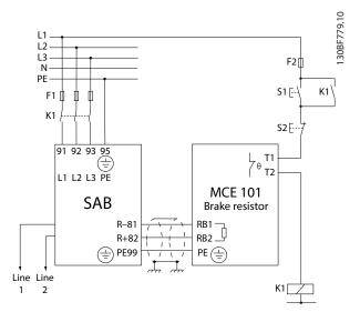
Illustration 2.14 Temperature Switch Disconnecting the Mains from the SAB
