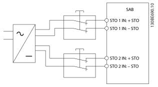
Illustration 2.10 Safety Relay with Plus and Minus Switching Output
