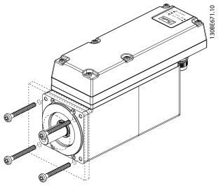
Illustration 6.21 Mounting of Size 2, 2.1 Nm Servo Drive
