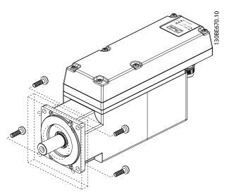
Illustration 6.20 Mounting of Size 1, 1.9 Nm, Size 2, 2.9 Nm, and Size 2, 3.8 Nm Servo Drives
