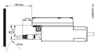
Illustration 6.36 Required Installation Distance and Minimum Bending Radius for M23 Angled Connector
