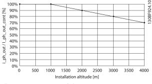
Illustration 6.19 Derating of Phase Output Current versus Installation Altitude
