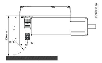
Illustration 6.35 Required Installation Distance and Minimum Bending Radius for M23 Straight Connector Angled connector
