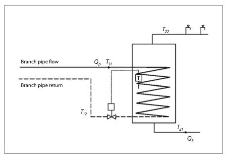
FIGURE 2: Storage tank unit, 110 litre volume, 17 meter of 3/8" coil installed
