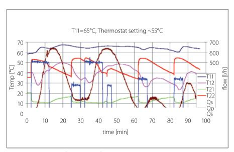
FIGURE 3: Example of tapping profile measurement applied on a 110 litre ST unit
