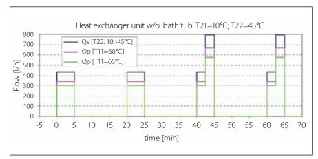
FIGURE 5: Heat exchanger hydraulic performance, heat exchanger type Danfoss XB06-1-34H
