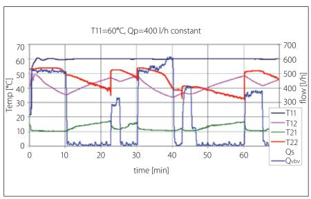
FIGURE 4: Example of tapping profile measurement applied on 110 litre ST unit, primary flow is constant
