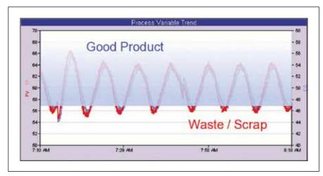
FIGURE 1: Oscillation in a process plant
