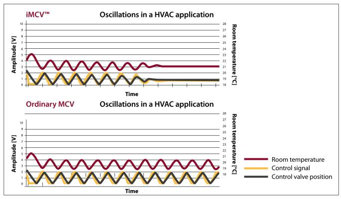
FIGURE 2: Oscillation in a HVAC application
